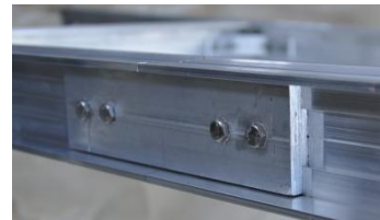
Beam Joint Detail (Double Clamped)
